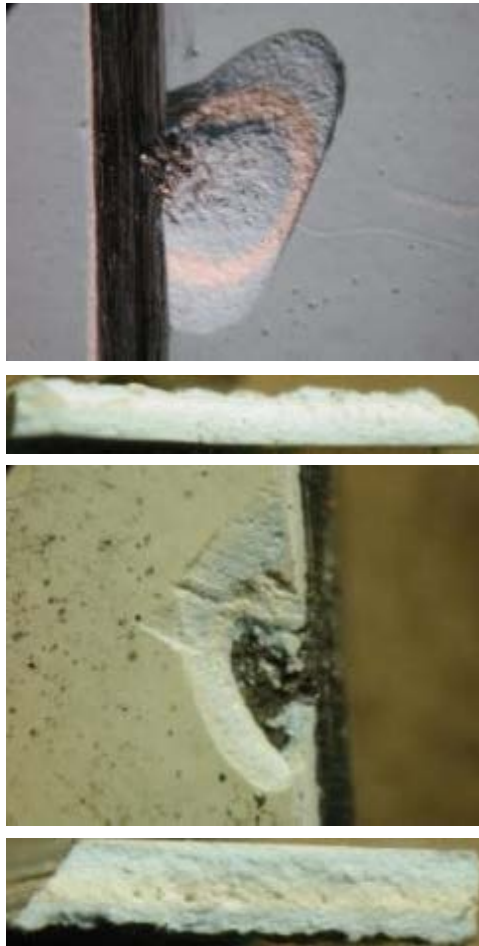
Figure 6a: Foam Results for 57 @ 40X Magnification (Top to Bottom: control, gas phase, hydrocarbon phase and aqueous phase)
