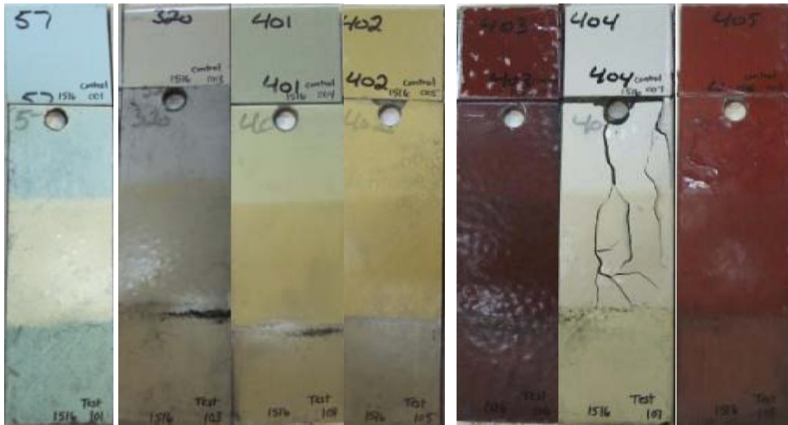
Figure 2: Autoclave Samples – After Exposure (Left to Right: 57, 320, 401, 402, 403, 404 and 405)
