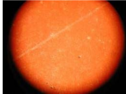
Figure 3e: Cracking Results - Panel 405 @ 40X Magnification (Left: gas phase, Right: hydrocarbon phase)
