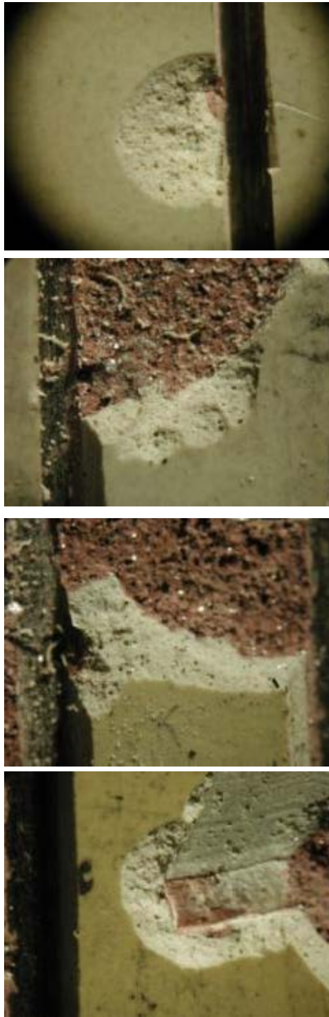
Figure 6b: Foam Results for 320 @ 40X Magnification (Top to Bottom: control, gas phase, hydrocarbon phase and aqueous phase)
