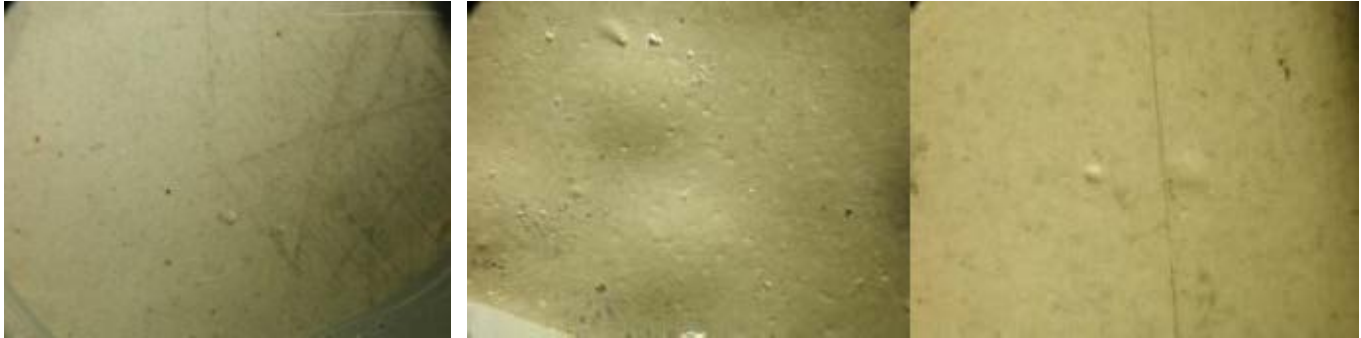
Figure 3b: Blister Results - Panel 320 @ 20X Magnification (Left to Right: gas phase, hydrocarbon phase, aqueous phase)
