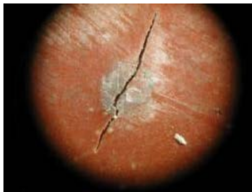
Figure 3d: Blister Results - Panel 405 @ 40X Magnification (hydrocarbon phase)
