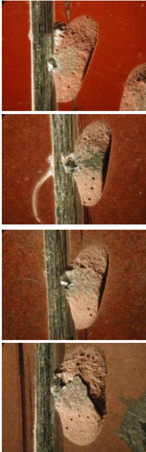
Figure 6e: Foam Results for 403@ 40X Magnification (Top to Bottom: control, gas phase, hydrocarbon phase and aqueous phase)
