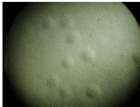
Figure 3a: Blister Results - Panel 57 @ 7.5X Magnification (hydrocarbon phase)
