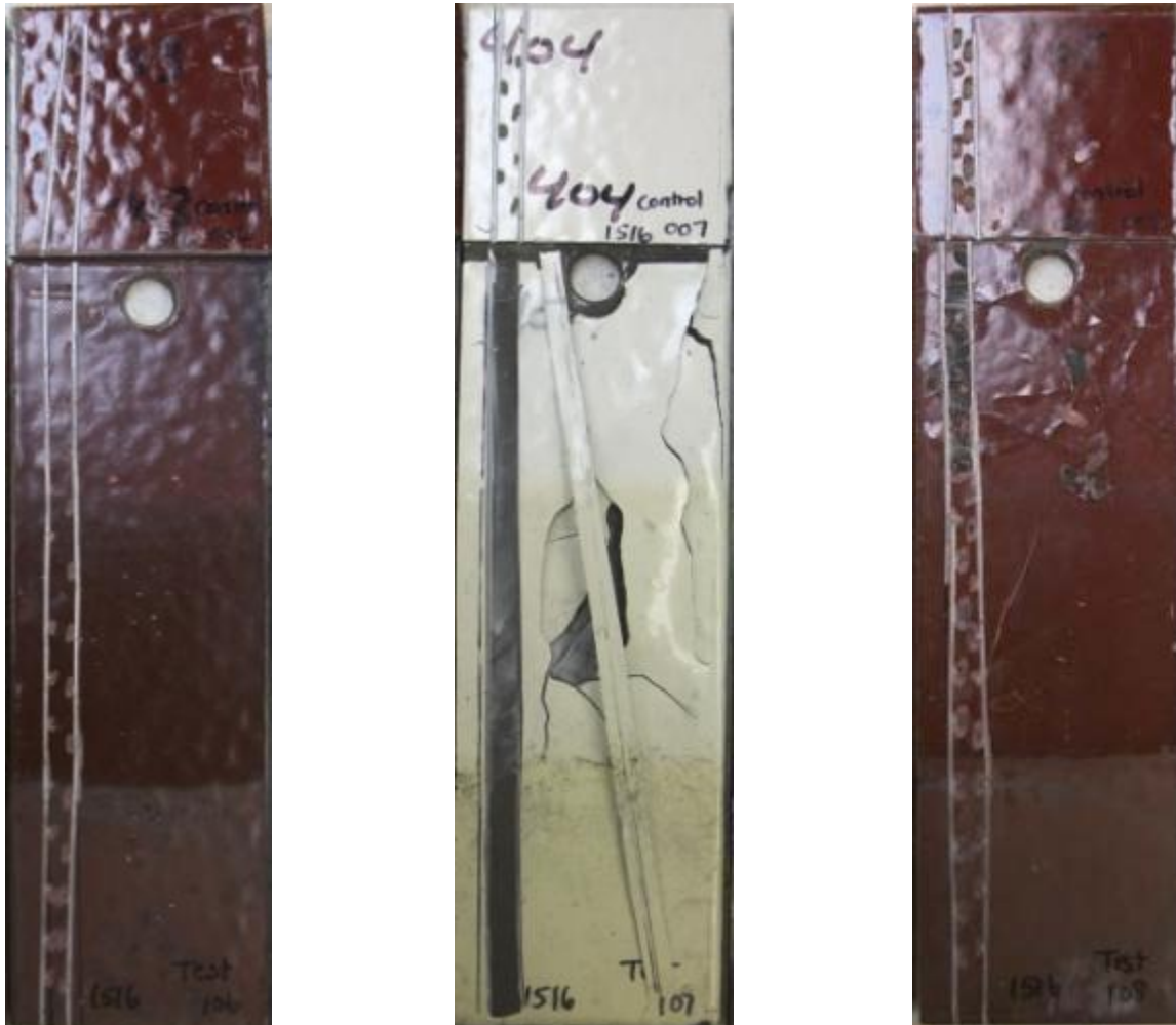
Figure 4b: Adhesion Test Results (Left to Right: 403, 404 and 405)
